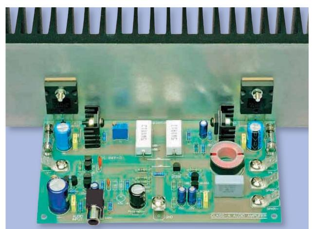
This life-size view shows the fully assembled left-channel amplifier module. Note that some minor changes were made to the PC board (just to the right of the audio input phono socket) after this module was assembled
