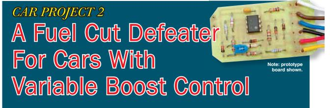
Are you intending to build the Variable Boost Control described earlier? If so, you will need to build this simple Fuel Cut Defeater (FCD) to eliminate the standard factory fuel cut, which typically occurs at boost levels of about 16 to 17psi. The unit is not adjustable, so no external controls are required.
