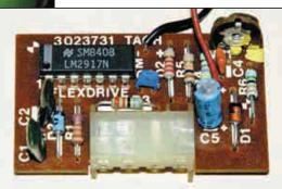
In essence, this tacho is a simple frequency-to-voltage converter driving a moving coil meter. The standard adjustment pot is shown top right.
