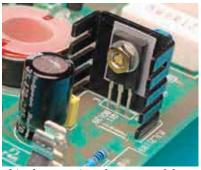
This close-up view shows one of the BD139 transistors (left-channel amplifier board). A second BD139 mounts on the other side of this heatsink.
