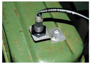
The reed switch was salvaged from an old film processor at the local tip. Here it can be seen mounted directly above the output pulley of the drill press.
