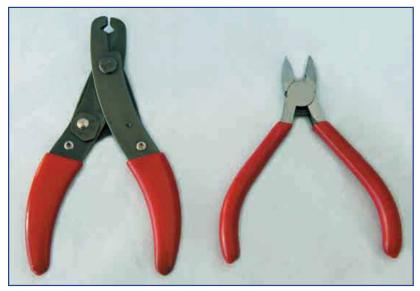
Fig.1. Proper wire strippers and cutters are essential tools for project construction, and an inexpensive combination tool (left) does both jobs quite well. It is also worthwhile augmenting these with a small pair of cutters (right) for intricate work and for cutting fine wires
