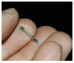
A reed switch from a speedo was initially used but some dummy bent a lead too close to the glass envelope and broke it! Another salvaged component was then used instead – the reed from a float switch.
