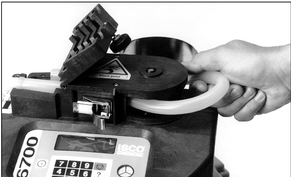
Figure 13 Removing and replacing the pump tube
