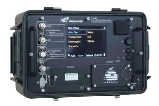
Full color display and easy to use front panel navigation utilizing a simple Joy-stick – The user friendly interface allows for fast and simple verification of aircraft installed avionic systems.
