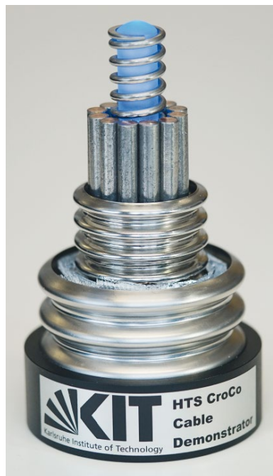
FIG. 7 This DC cable model with high-temperature superconductors of the 100 kA class at 20 K has an outer diameter of only 70 mm.
