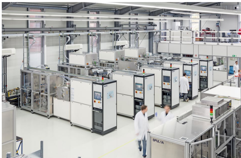
Fig. 1 Production facilities for manufacturing HTS tape conductors at THEVA Dünnschichttechnik GmbH in Ismaning near Munich.
