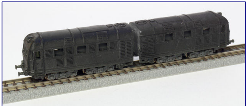
In the DB's double diesel locomotive V 188, the details of the body are much more apparent in the resin printing.
