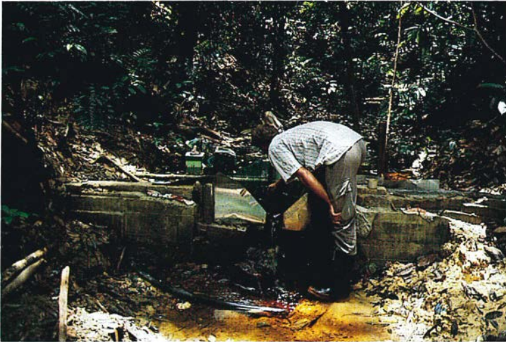
Calibration of a dam with V-notch in the experimental catchment.
