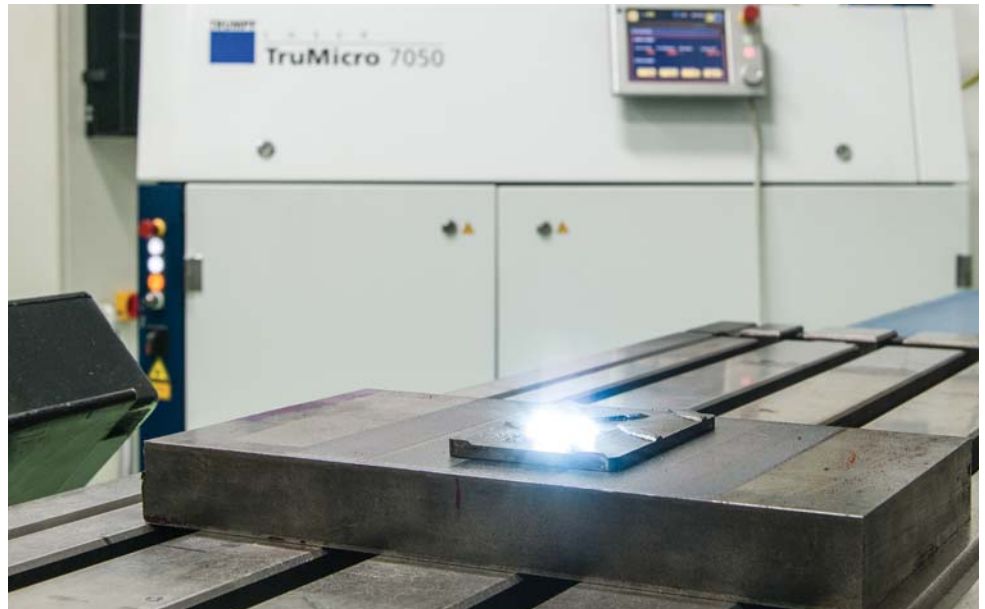
Joining Technologies uses a TruMicro laser to clean customer parts.
