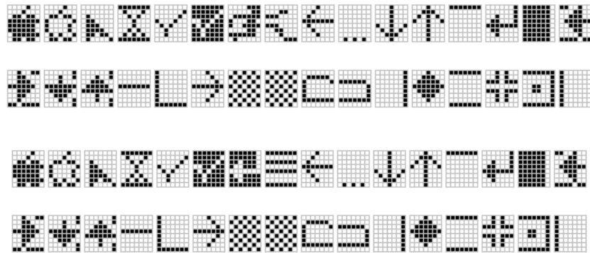
Figure 1. MouseText as implemented on the Apple IIc (above, with RUNNING MAN) and IIGS (below, with replacement characters). (Wikipedia)
