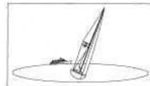
Fig. 3. Test orientation for a "heeled" reflector (catch rain position shown).
