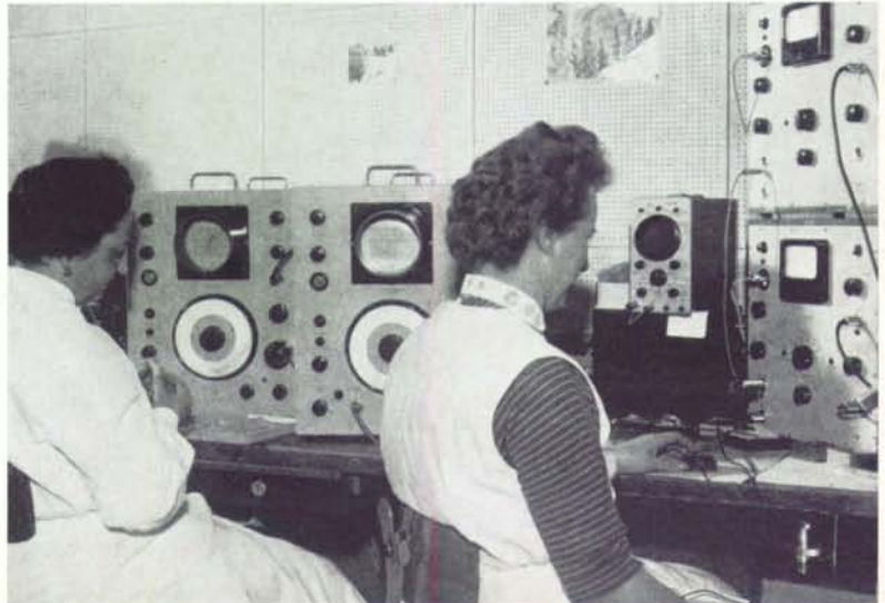
Fig. 8 Set-up of a testing arrangement for production control of hearing aids with visual check on frequency characteristics
