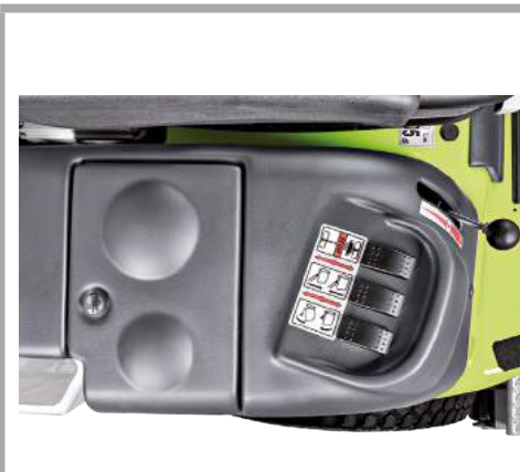
Controls via electric buttons
