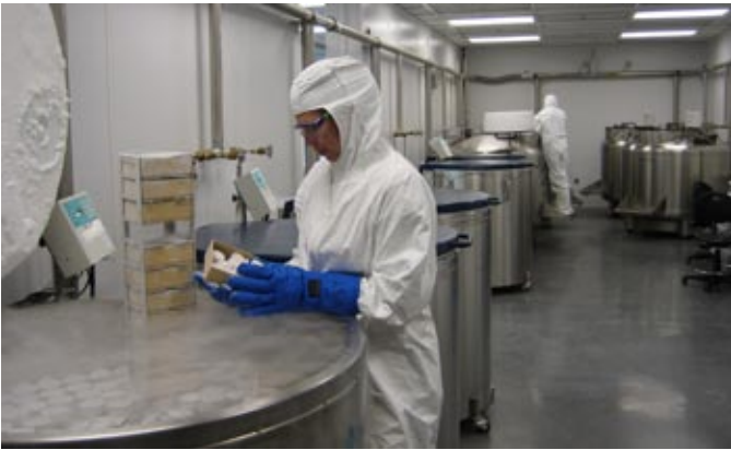
Removing samples from a liquid nitrogen vapor phase freezer in the Marine Environmental Specimen Bank maintained by NIST. Photo Credit: R. Pugh
