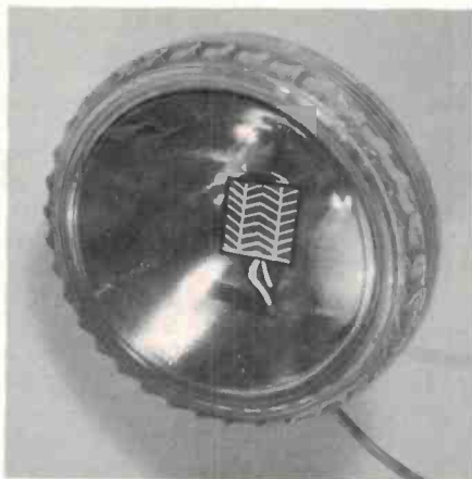
Close up of our receiver input device. This consists of a small solar cell piece mounted in a reflector taken from a 'Dolphin' lantern. To mount the cell, we cut a slot in one side of the reflector, put Silastic on the rear of the solar cell (leads already attached) and inserted it in place. It proved very effective.
