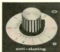
Anti-skating system of Dual 1209 and 1219 has separate calibrations for elliptical and conical styli.
