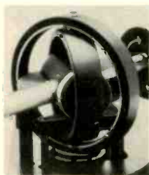
Twin-ring gimbal system of Dual 1219. Arm pivots vertically from inner ring, horizontally from outer ring. All four suspension points have identical low-friction bearings.
