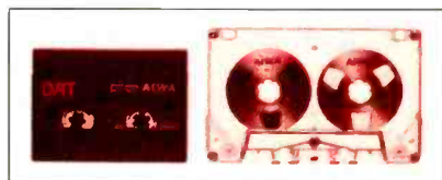
The DAT cassette is about half the size of a conventional analog tape cassette.
