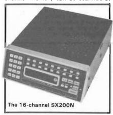
two rates — Fast (8 channels per second) or Slow (4 channels per second). Similarly, there are two Seek rates — Fast (10 channels per second) and Slow (5 channels per second). Again, an internal whip and speaker is fitted, its audio output is 2 watts and its
