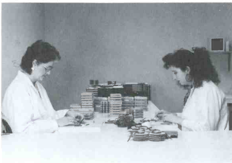
Once cleaned and dried, new pressure pads, brake pads and washers are inserted in the shell.
