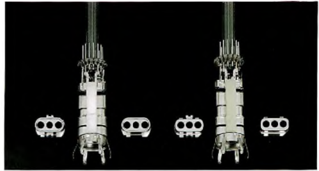
Fig.4 Standard electron gun with circular apertures (right) and polygon gun (left) with apertures configured to compensate the non-radially symmetric field generated by the lens formed by the oval ridge
