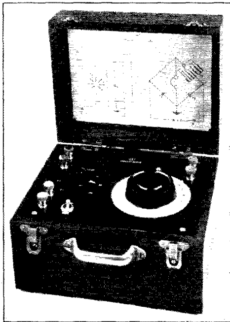
THE CAPACITY BRIDGE OPEN FOR USE
