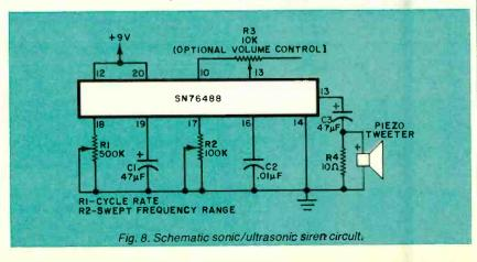
The cycle rate can be varied from a few tenths of a hertz to several hertz by altering R1's setting.
