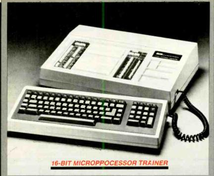
The Model ET-100 Learning Computefrom Heathkit/Zenith Educational Systems is an 8088-based trainer, 16-bit computer, and engineering design and test system all rolled into one. Its standard features include a solderless breadboarding system that provides direct access to all address, data, control. and I/O lines, and four voltage supplies detached typewriter-style keyboard, 32K of ROM programmed with a CP/M asserbler, screen editor, and Circle No. 37 on Free Information Card
