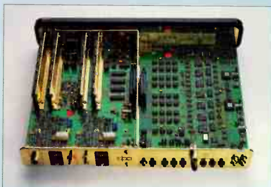
Surface mount components make it possible to get the thousands of components into one case.
