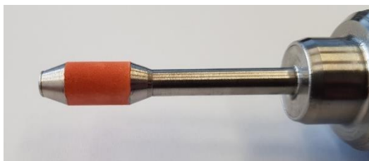
Figure 1: Resonator with fouling model (copper deposit).
