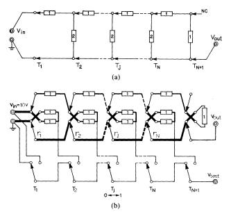
Fig. 2. (a) An *N*-bit Cutkosky voltage divider with cascaded DPDT switches  $T_j$ , each drawn as a pair of interchangeable contacts. With all switches at zero (as shown), all horizontal "dropping resistors" appear in the upper branch. Resistance values indicated are relative to  $R_{nom}$ . (b) Wiring diagram for the same divider. Heavy links identify the requisite low-resistance connections. Additional SPDT switches give access to internally generated  $V_{test}$  for self-checking purposes.
