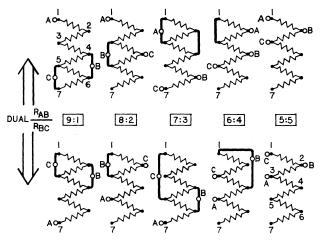
Fig. 3. Dual configurations of networks (after Thompson [5]) producing resistance ratios for each step of a single-decade divider. Network has six nominally equal resistors connected in series. Thick lines represent shorting links.
