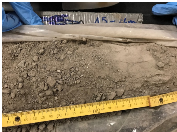
Bohrkern: 4–5 m: Helles, pulvriges Material.
