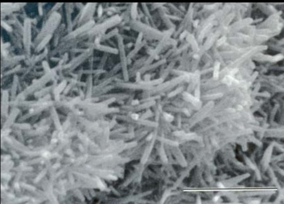
Halloysite formation on weathering biotite in granite-gneiss saprolite
