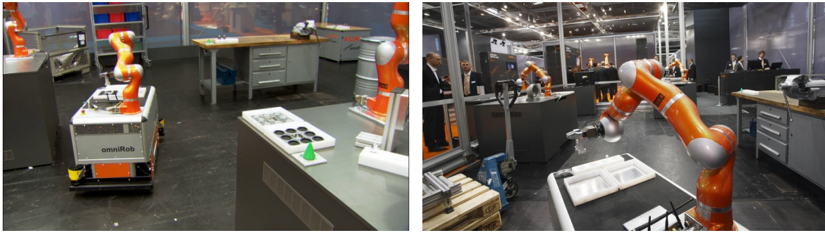
Figure 2.24: The omniRob navigating with the proposed trajectory generation approach in an industrial mobile manipulation demonstration at the KUKA booth at the AUTOMATICA 2010 fair.
