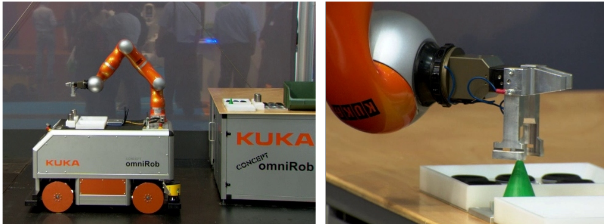
Figure 3.1: An autonomous platform drives to a work station and docks to it, relying only on its safety laser scanners. The positioning accuracy is high enough to carry out subsequent manipulation actions.
