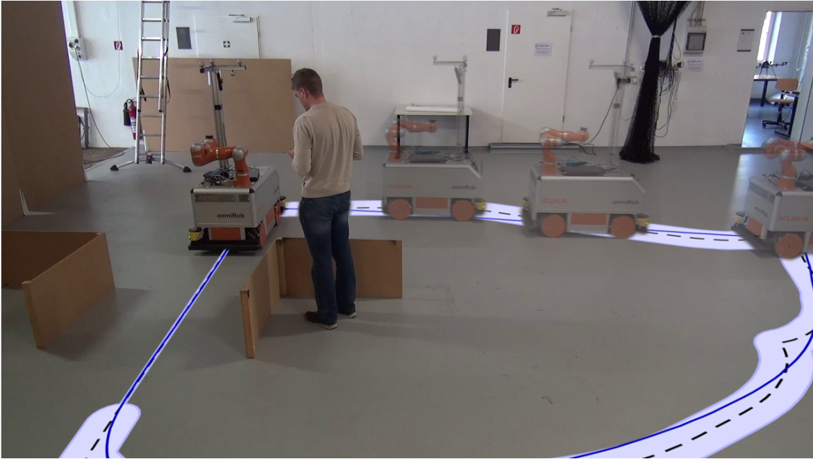
Figure 5.11: Extending our framework to teach-optimize-repeat for omnidirectional robots: We optimize the user demonstration (dashed line) within variable, user-defined bounds (shaded area) to obtain a smoother and faster execution (solid line).
