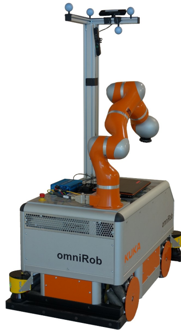
Figure 2.12: The omnidirectional mobile manipulator omniRob by KUKA that we used in our experiments.
