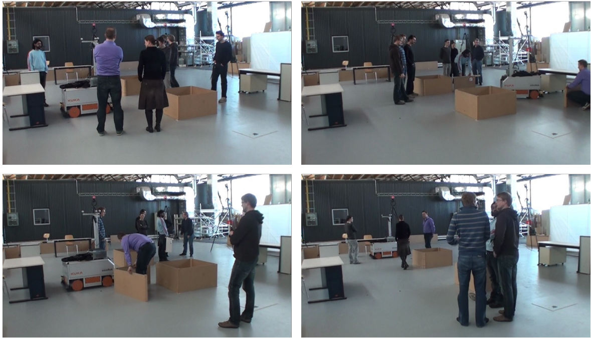
Figure 3.5: Experiment with the omniRob in a dynamic environment in which people and wooden boards changed the appearance of the environment. Figure 3.6 shows the results for different levels of environment dynamics.
