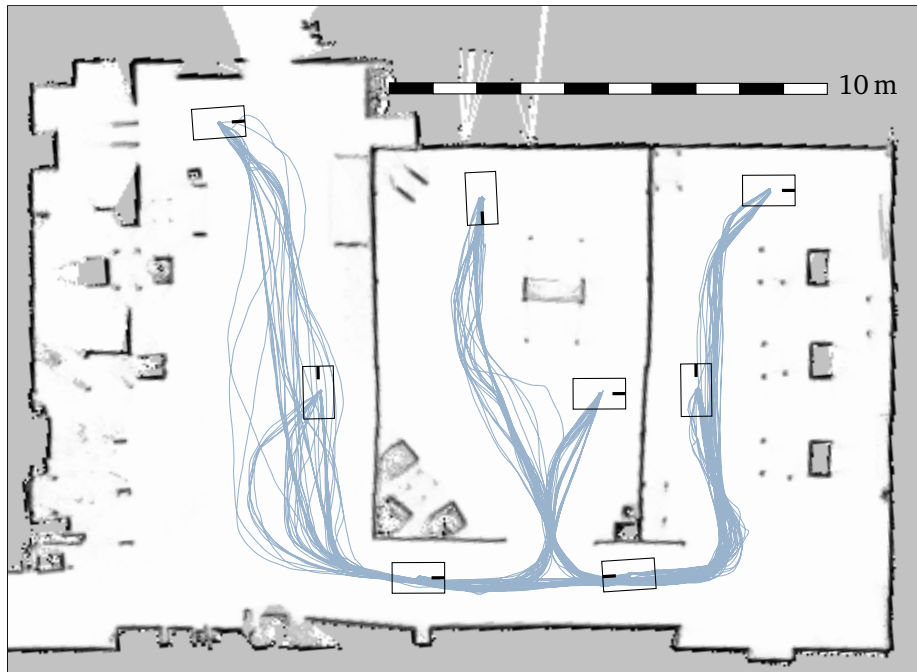
Figure 2.22: Our experiment for navigation in a dynamic environment. The robot looped for 2.9 km and two hours between eight goal configurations while object rearrangements and moving people changed the environment. The figure shows roughly half of the driven paths, deviations from the typically chosen route are due to dynamic obstacles blocking the usual path of the robot.
