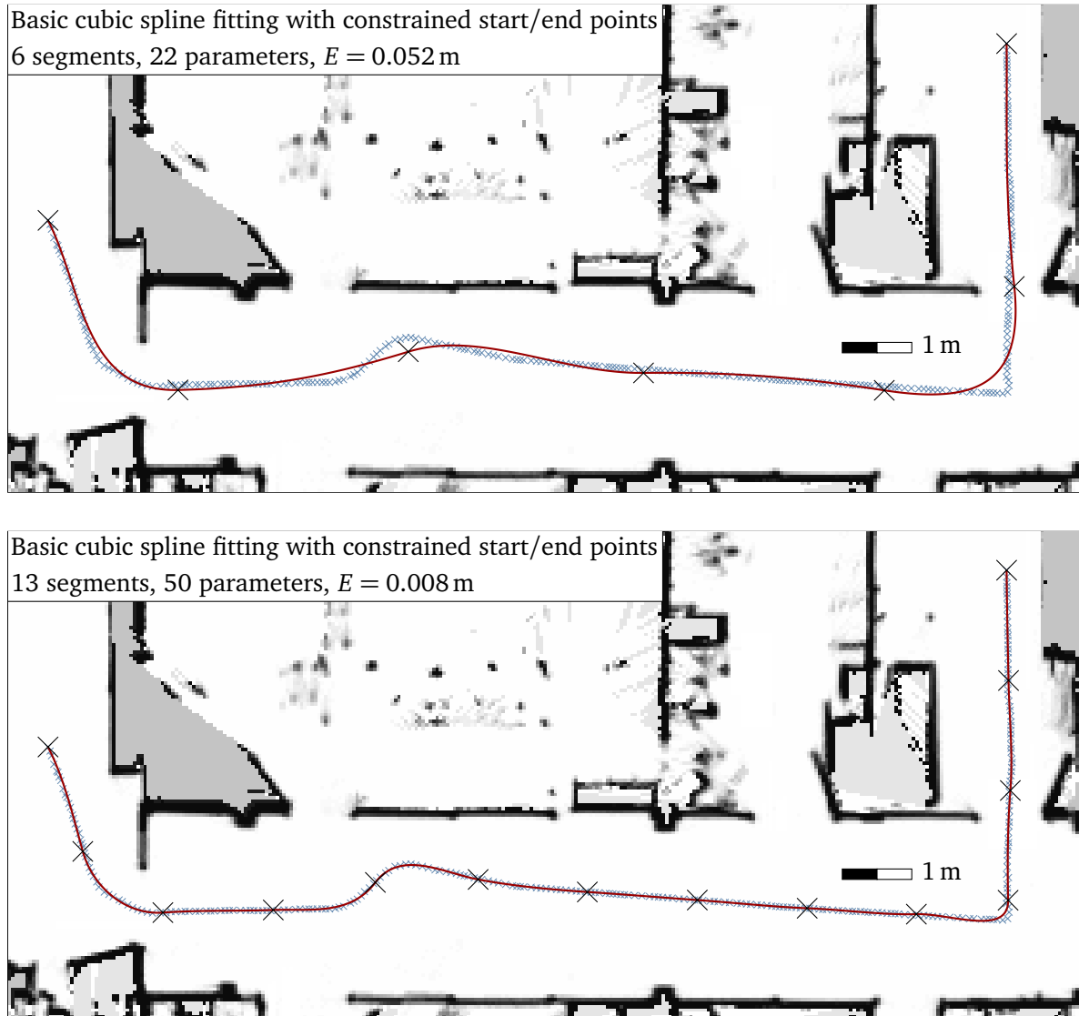
Figure 4.2: Linear least-squares fitting of cubic splines with constrained start/end points. With 22 parameters (top) this overly smooths the corners, causing a high residual error. With 50 parameters (bottom) the error is comparable to our method with 23 parameters, as shown in Figure 4.1.
