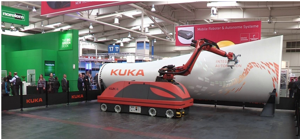
Figure 2.1: The KUKA Moiros robot using our system for accurate omnidirectional navigation during a demonstration at the Hannover Messe 2013 fair. Our system accounts for platform and safety constraints and reliably navigated for several days in this inspection task for wind turbine blades.
