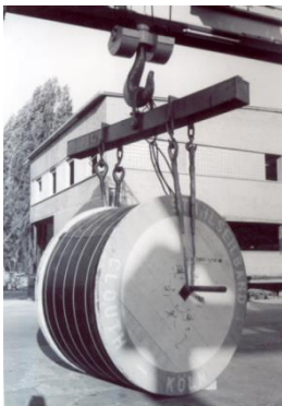
Conveyor belt transport onto lorry
