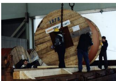
Loading of "Conti-Tech-Clouth" conveyors
