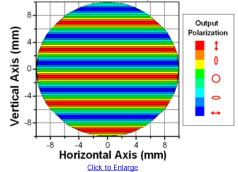
Figure 2. False-color plot of a calculation showing a linearly polarized input beam parallel to the optic axis of the thick wedge after passing through the depolarizer.
