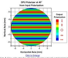
Figure 4. False-color plot of a calculation showing a linearly polarized input beam parallel to the optical axis of the thin wedge after passing through the depolarizer.
