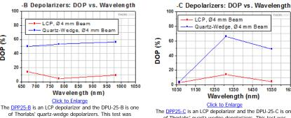
The DPP25-C is an LCP depolarizer and the DPU-25-C is one of Thorlabs' quartz-wedge depolarizers. This test was
