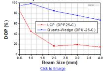
The DPP25-C is an LCP depolarizer and the DPU-25-C is one of Thorlabs' quartz-wedge depolarizers. This test was performed using a 1310 nm MCLS1-1310 laser diode module (1 nm FWHM bandwidth)
