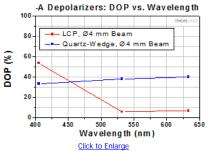
The DPP25-A is an LCP depolarizer and the DPU-25-A is one of Thorlabs' quartz-wedge depolarizers. This test was performed at three wavelengths using three different lasers
