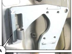
7.) Please mount the LSD chassis plate with screws (A) on the new fitting points of the hinges.
