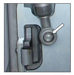
17.) Carefully pivot the door up and hang in the gas spring at the fitting point of the chassis plate. Secure it also with the supplied security ring.
