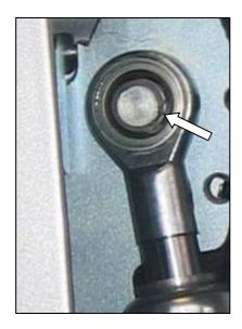
16.) Hang in the gas spring on the fitting point of the swing arm. Secure it with the supplied security ring, by means of needle-nosed pliers.
