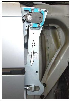
12.) Adjust the height of the door by vertical movement of the chassis plate.
