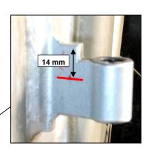
4.) The LSD chassis plate has to be mounted at the fitting points of the original hinges on the chassis (A-pillar).
