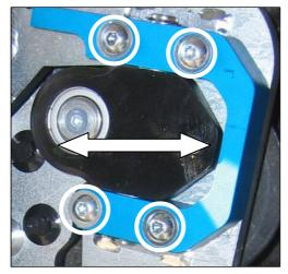
11.) Fix the swing arm to the chassis plate with Allen bolts (4x) and adjust the door via moving the swing arm to chassis plate adjustable connection mount with horizontal door gap adjuster.
