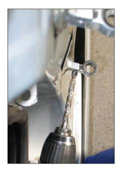
6.) The hinges have to be drilled and reworked with a tap on the points shown in the picture above.
