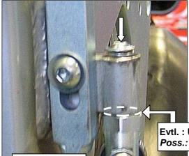
8.) On the upper original hinge on the A-pillar you will have to mount the slide roller with a socket screw (M6x35 or M6x40 + ring washer) so that you have a distance of 2 mm between lower edge of the slide roller and upper edge of the swing arm.
