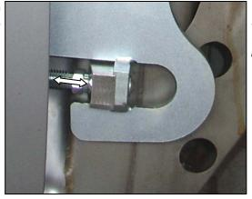
14.) Position the adjustment screw (1) in that way, which the door closes in the middle position.
