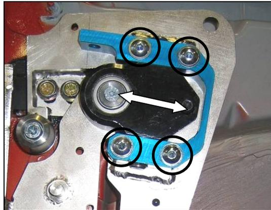
12.) Fix the swing arm to the chassis plate with Allen bolts (4x) and adjust the door via moving the swing arm to chassis plate adjustable connection mount with horizontal door gap adjuster.
