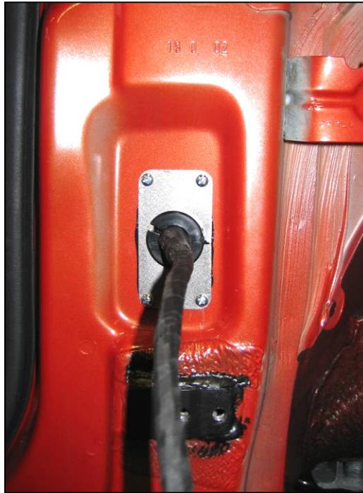
5.) Close the original cable tree lead-through with the supplied cover plate (required drilling: Ø 2mm) and possibly it can be sealed additionally with chassis glue.
