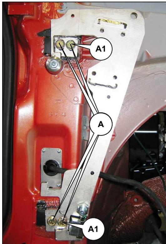
7.) Now the LSD chassis plate has to be mounted at the new mounting points with screws (A). Mount the supplied balancing washers under the chassis plate at point (A1).
