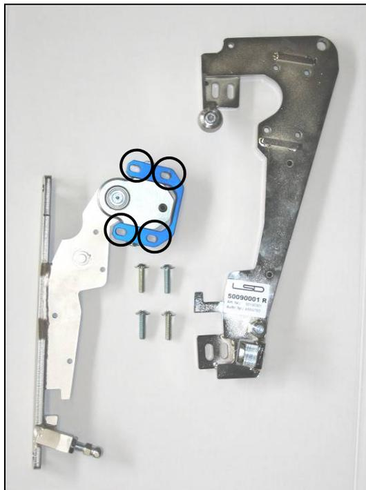
6.) Dismantle the swing arm off the chassis plate.
