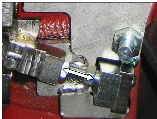
14.) Position the adjustment crew (1) in that way, which the door closes in the middle position.
