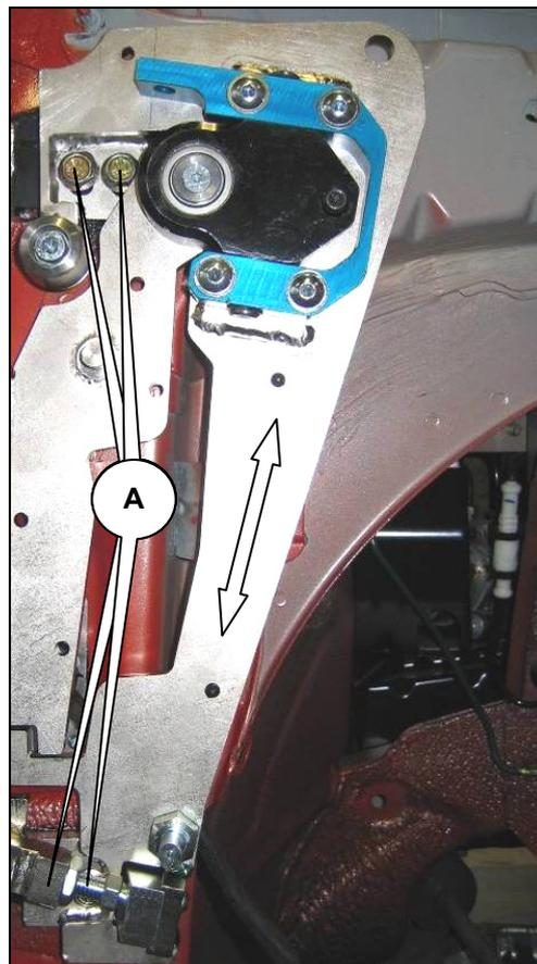
13.) Adjust the height of the door by vertical movement of the chassis plate.
