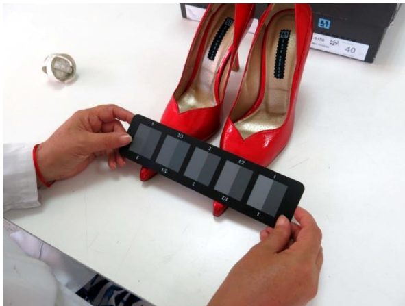
Fig. 4: Grey scale to check colour variations between the confirmation sample and the manufactured samples
