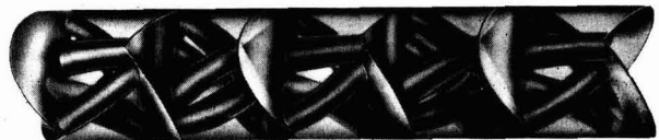
The interior of an AMK/Ross motionless mixer
