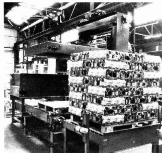
Lo-Stak Mk II palletising system for handling unit loads
