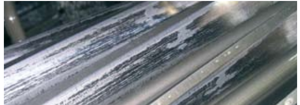
Picture 01: Strong micro-pitting and pitting on tooth flanks
