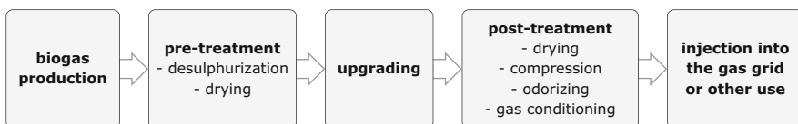
Fig. 8.7 Schematic diagram of the biogas upgrading process
