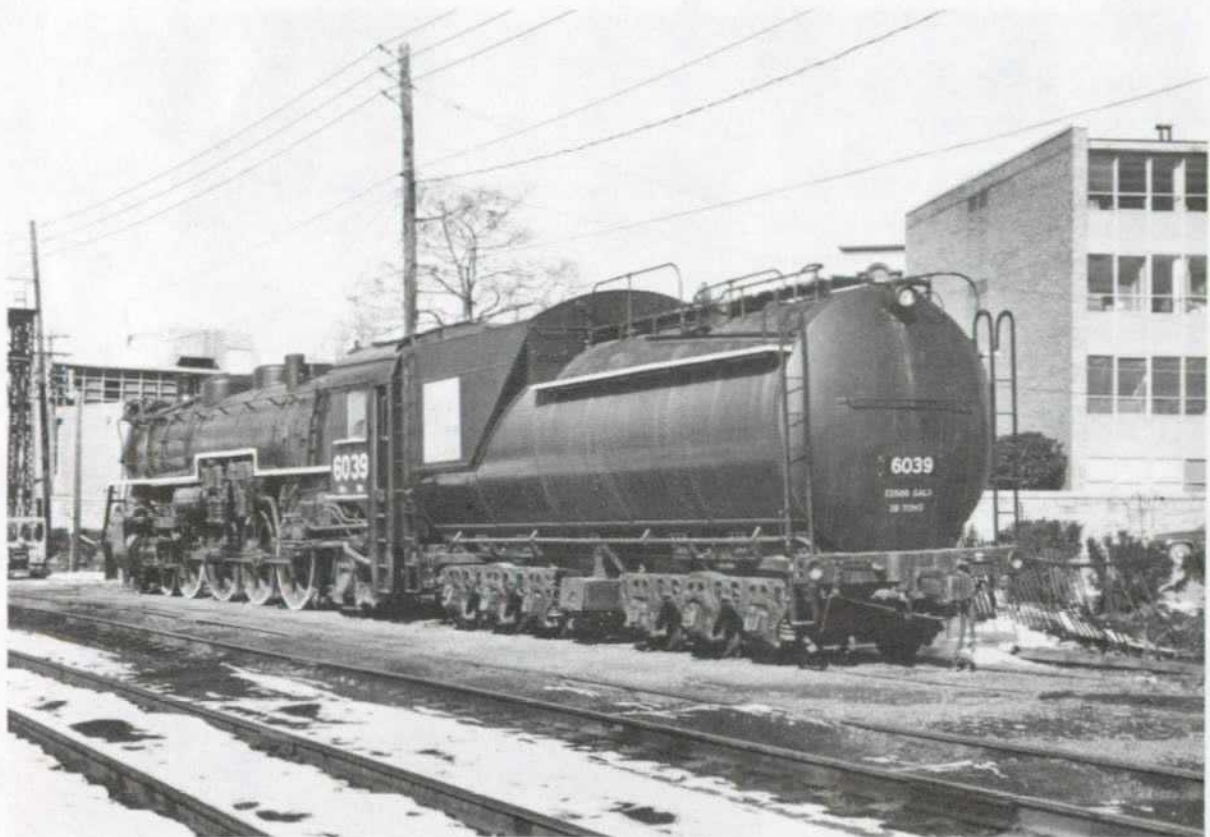
The distinctive cylindrical tank of a Vanderbilt tender graced Grand Trunk Western Locomotive No. 6039, the only tender of this type in the Steamtown Foundation collection.
