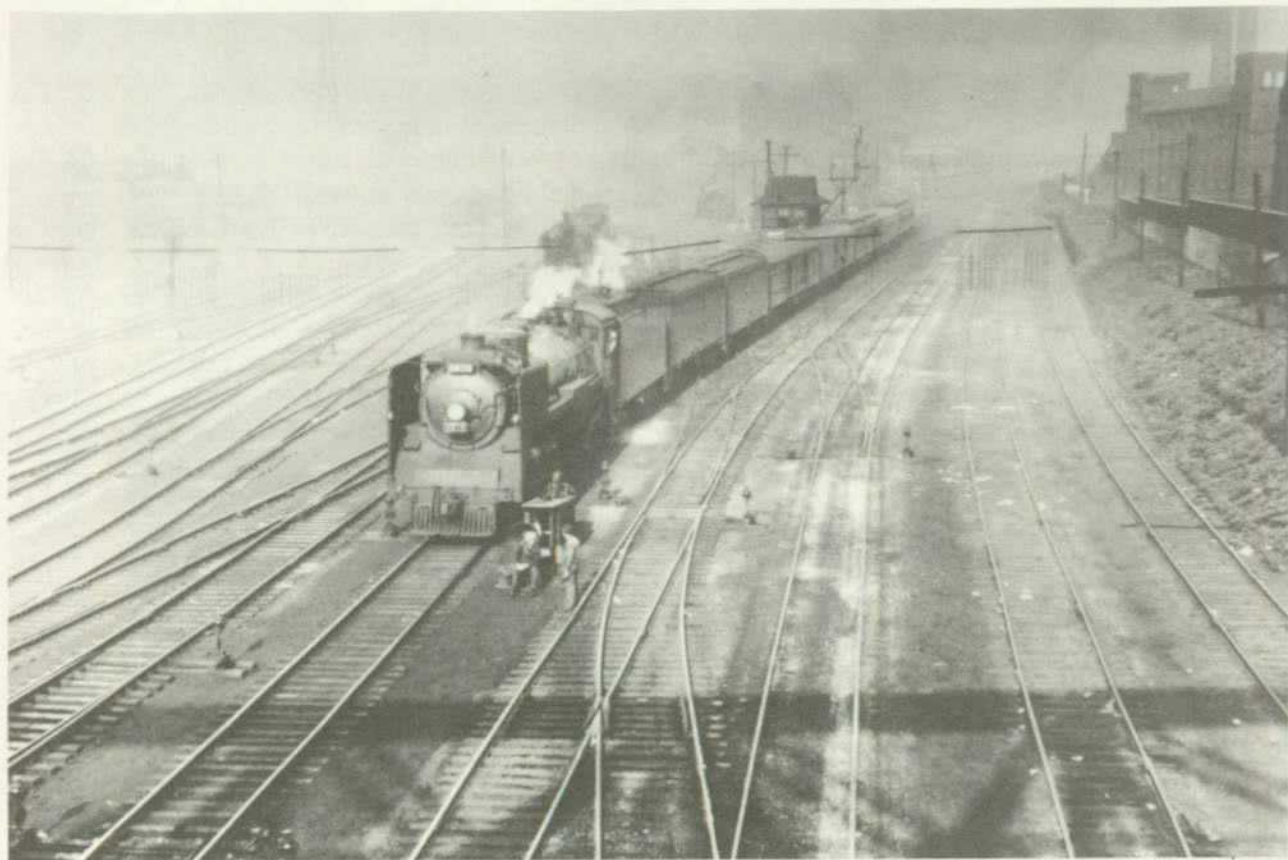
Canadian Pacific Railway Locomotive No. 2816 arriving at Toronto, Ontario, on July 9, 1948, with eastbound Train No. 8. Note the smoke deflectors or "elephant ears" alongside the smokebox, which are no longer on the locomotive.
