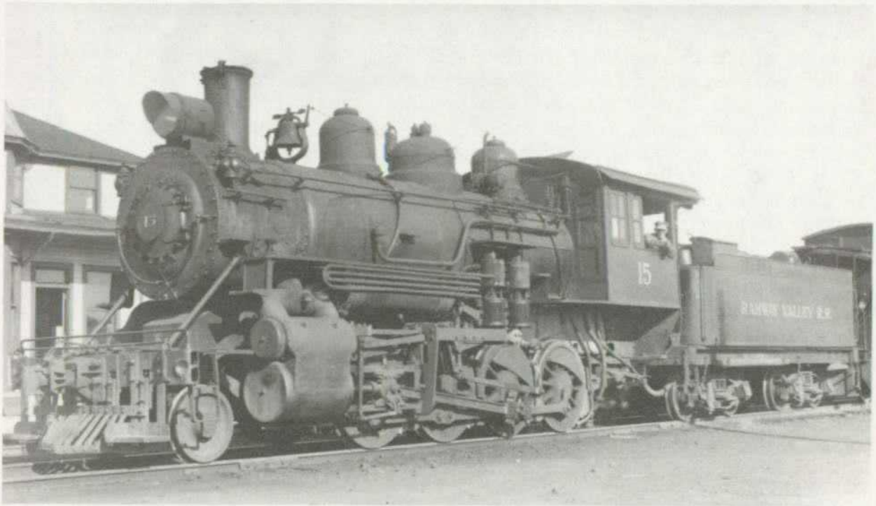
Rahway Valley Railroad Locomotive No. 15 featured a front number plate and a headlight mounted on top of the smokebox, which make her look different from her present appearance in Scranton, Pennsylvania.
