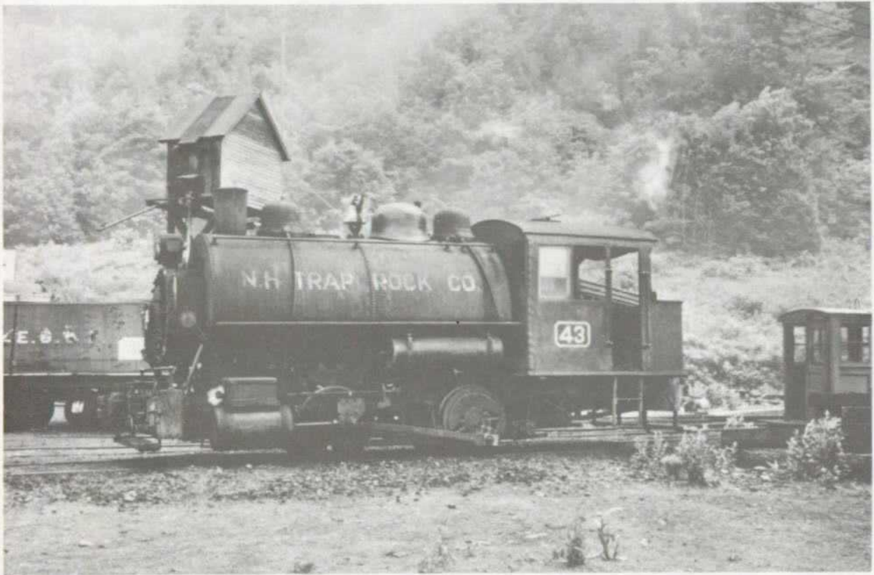
Edgar T. Mead's photo of No. 43 illustrated its "New Haven Trap Rock Co." lettering and the number on the side of the cab (above). New Haven Trap Rock Company 0-4-0T Locomotive No. 43 (below).
