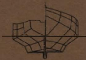
Figure 80 *Katrina*. German "ewer" type fishing ketch of the lower Elbe, circa 1870. Note straight line section double-chine hull form with dagger board. The lower part of the hull was a fish tank or wet well
