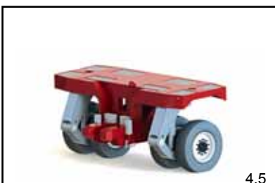
1-axle dolly trailer with front and rear hook coupling
