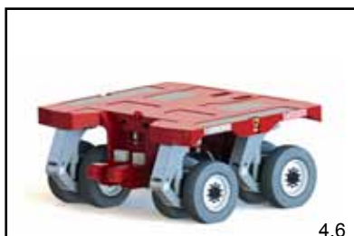
2-axle dolly trailer with front and rear hook coupling
