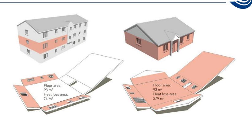
Figure 3 'Unfolded' structures with their heat loss areas shaded orange. End mid-floor apartment (left), bungalow (right)
