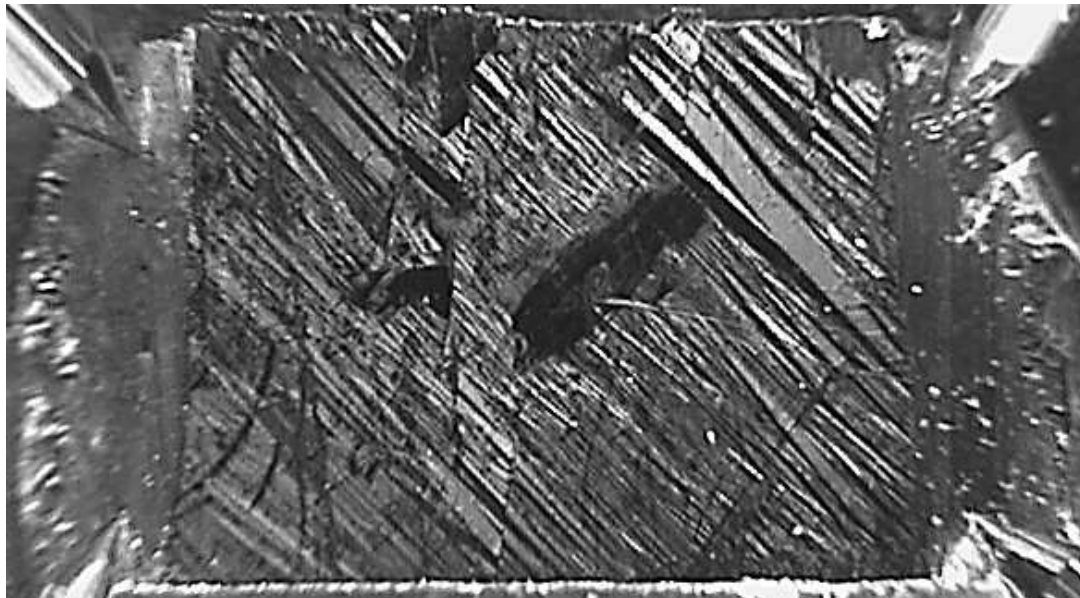
Figure 7.9: Micrograph showing the Ni 63 Al 37 sample surface in the martensitic phase. The surface relief, originating from the self-accommodation process, is highly oriented.
