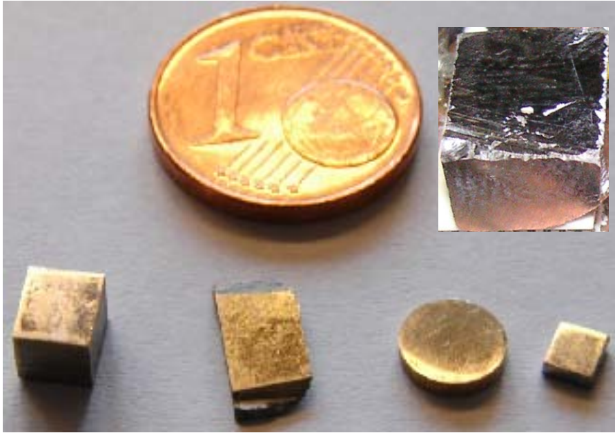
Figure 7.8: Photograph showing the analyzed samples in their parent phase at room temperature and a 1-eurocent coin as a reference. From left to right: \text{Au}_{50.5}\text{Cd}_{49.5} , \text{Ni}_{63}\text{Al}_{37} , \text{Cu}_{68}\text{Zn}_{16}\text{Al}_{16} (which will serve as a reference in section 8.5 and in the introduction of chapter 8), and \text{Fe}_{68.8}\text{Pd}_{31.2}^{\text{single}} (both the single crystal and the polycrystal have identical shapes). In the upper right corner a photograph of the \text{Ni}_{52}\text{Mn}_{23}\text{Ga}_{25} sample has been added according to scale.
