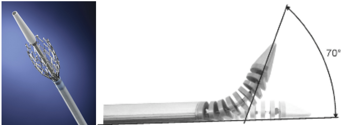
Figure 3.26: Two applications of the shape memory effect: A stent used in medical engineering (left) and an adaptive winglet as part of an aircraft (right).
