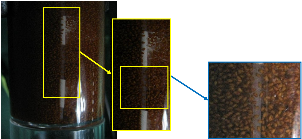
Figure 5.14 : Visualization of the hypothesis of shear induced particle migration using “Khakshir” particles in water.
