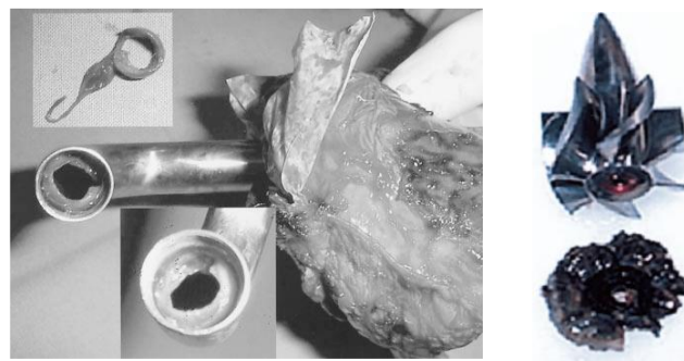
Figure 3.5: Thrombus formation in the different parts of MicroMed DeBakey VAD [52]
