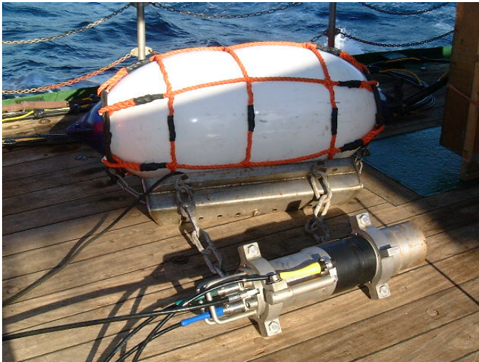
Figure 6.2.2.1: GI airgun with gun hanger and floatation.
