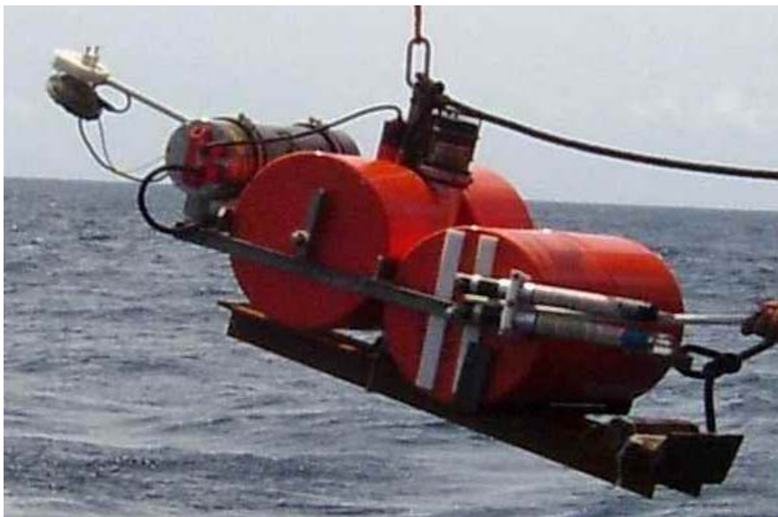
Figure 6.2.4.1: Ocean-Bottom-Seismometer – OBS - during deployment.
