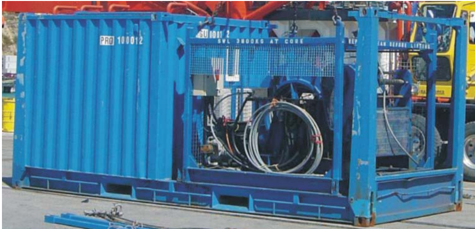
Fig 6.6.1: Deck-container with winch and the control unit, also used for storage of boxes and the TMS + ROV during transport.
