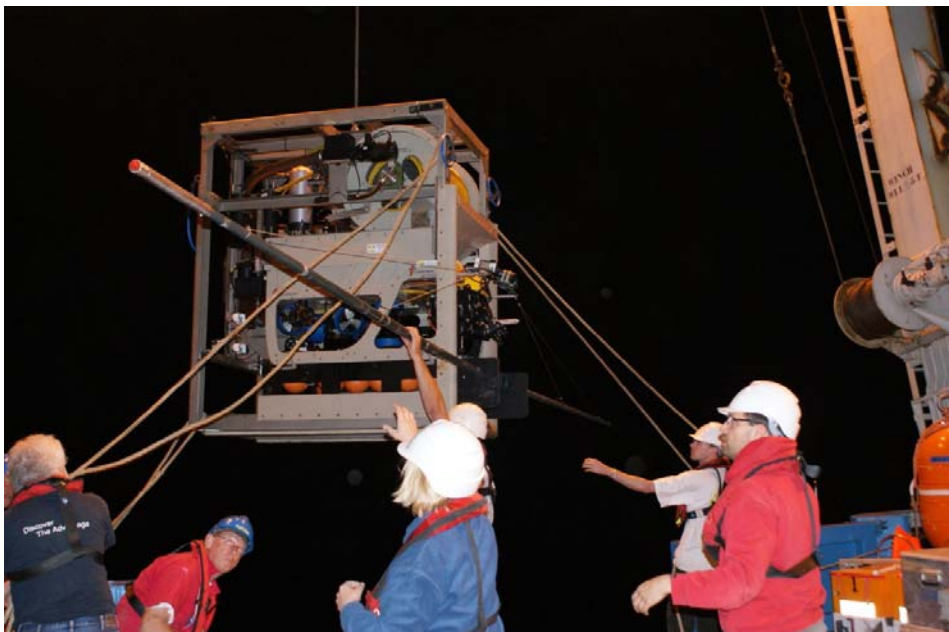
Figure 6.3.1.1: Upper panel: Hybrid marine EM receivers capable of recording low-frequency electric and magnetic field data as well as high-frequency electric field data. Bottom Lower panel: Deployment of 10-m electric dipole transmitter mounted on ROV for the active source EM experiment.
