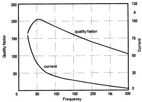
Fig. 1:Quality factor and current vs. frequency for a resonant test system 80A, 254kV, no. 7, 8 in table 1
