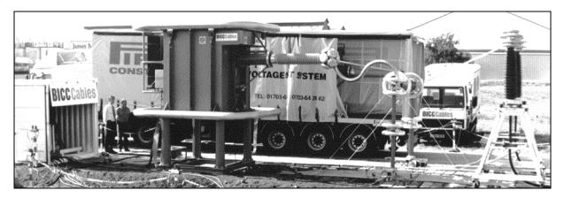
Fig. 3: Parallel connection of two identical test system 90A, 150kV to extend the available test current to 180A (By courtesy of BICC Cables Ltd., U.K. and Pirelli Construction Company Ltd., U.K.)
