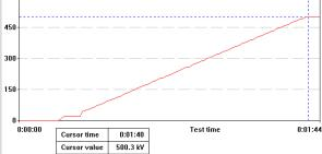
Fig. 5: Records for searching resonance frequency, (upper screen) and following voltage rise (lower screen)
