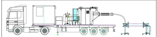
Fig. 2: Frequency-tuned resonant test system 90 A, 150 kV on a trailer with HV filter for PD measurement
