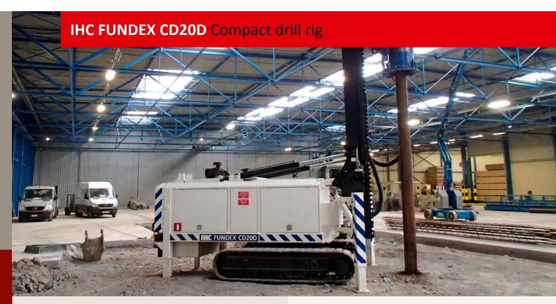
The IHC FUNDEX CD20D is a compact foundation machine for making various drilled piles in places where space and height is limited.
