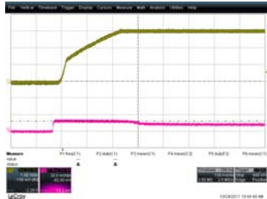
Figure 4: input and output voltage during startup of the converter
