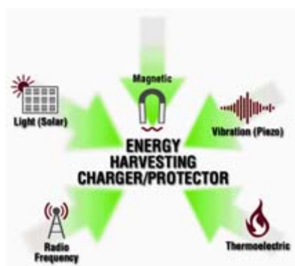
Figure 1: Energy harvesting uses unconventional sources to power circuitry
