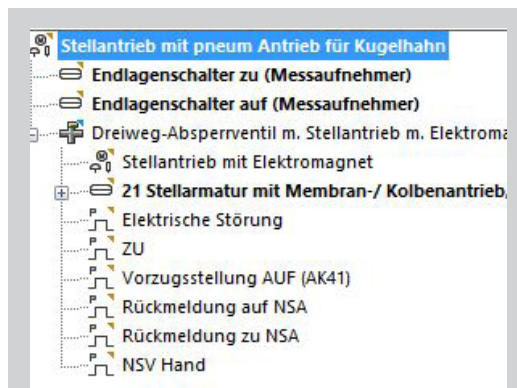
This logical structure (valve view) created in step 3 is visible in the CADISON® Tree
