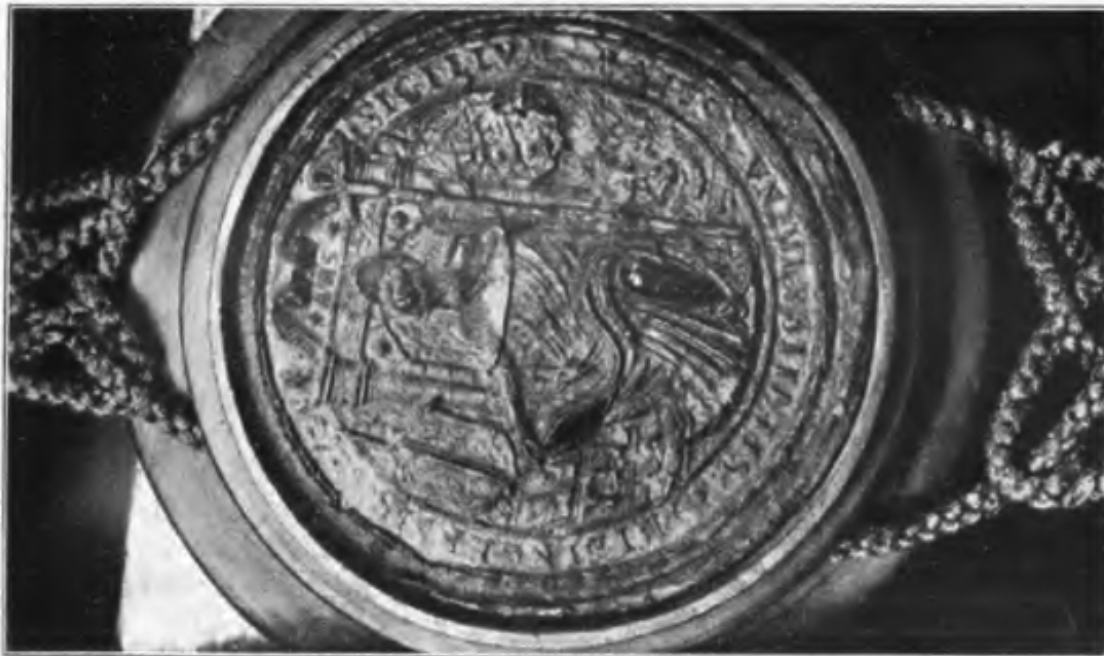
Receiving 541 of a red seal of the former University of Dillingen with ordinary silver-bromide plate. Recording II with a panchromatic plate and orange filters. It would be expected that the image II would at least provide an equally high-contrast image as image I. - Experiments with other plates and optical filters have brought no better results than image I.
