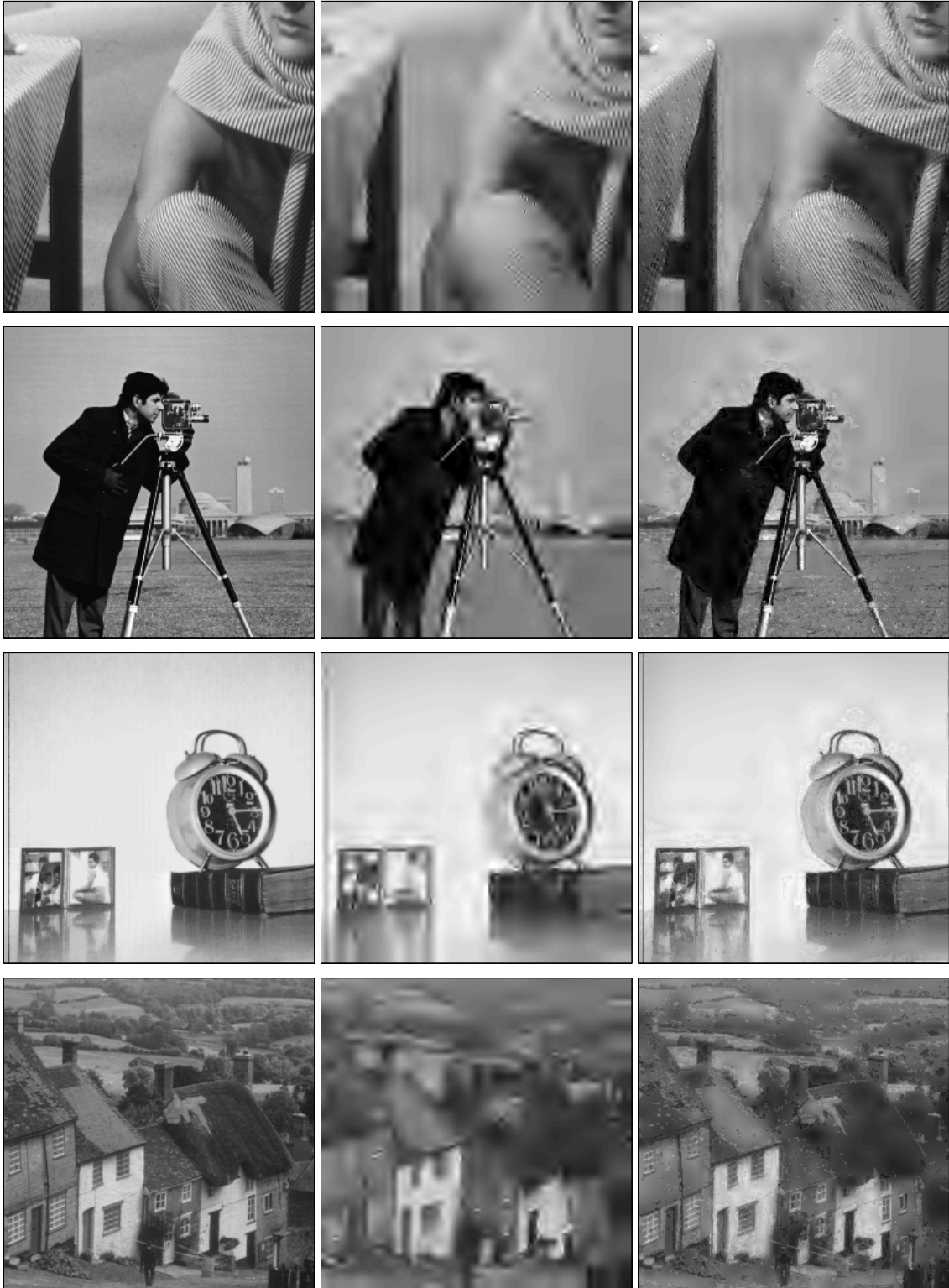
Figure 3: (Left) Original image; (middle) tensor product wavelet transform with 9/7 filter, keeping only 500 nonzero coefficients (nzc); (right) our hybrid method with 9/7 filter, keeping only 500 nzc.
