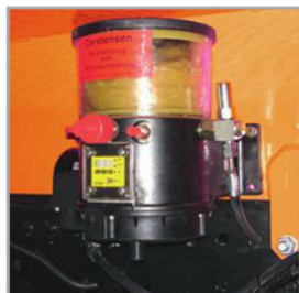
Central lubrication unit
