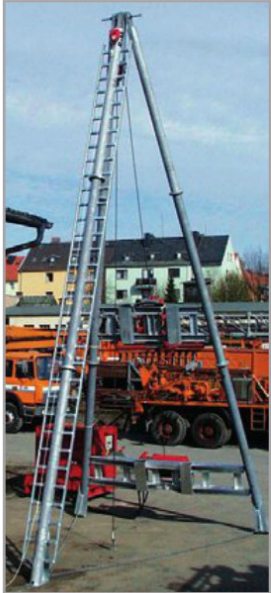
Three-legged trestle with striking mechanism and winch for the education of well borers in Rostrup (Bau ABC)
