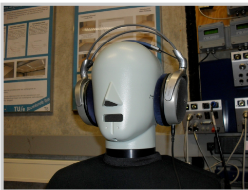
Fig 5. Headphone transfer measurement using a HATS.
