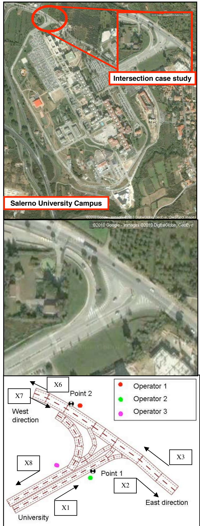
Fig. 4: Case study: a) Salerno University Campus with; b) Zoom on considered intersection; c) Implementation of the intersection in CadnaA, with measurement points and operators position.
